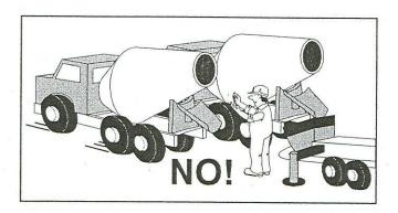
**3.2 WARNING! CRUSHING HAZARD.** Do not get closer than 10 feet to the concrete pump, concrete pump trucks, and/or crane lift bucket unless you have a clear view of the spotter who is directing you. If you lose sight of the spotter, stop immediately. Do not continue to back up until line-of-sight has been re-established.
