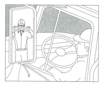
**3.4 WARNING! CRUSHING HAZARD.** If you find yourself acting as the spotter for another concrete delivery vehicle, make sure the driver of the concrete delivery vehicle is watching you. Make sure you're not in the path of the concrete delivery vehicle as it backs towards the hopper.
