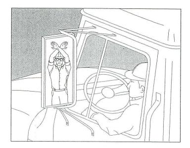
**3.3 WARNING! CRUSHING HAZARD.** When backing towards the concrete pump, concrete pump trucks, and/or crane lift bucket, the spotter must use clear and concise hand signals. Agree on hand signals before you begin the back.
